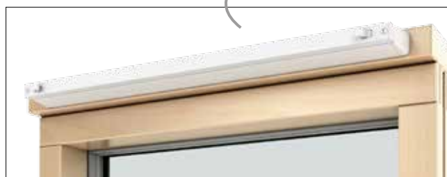
Acoustic trickle vent. The vent is machined into a timber packer with an external aluminium profile in the same colour as the window sashes. Documentation on air flow can be requested. Achieves a sound reduction value of D_{n,e,w} 40 dB.
