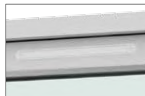
Click vent. For outward opening doors only. Natural anodised surface finish. Free ventilation opening 4000mm 2 . Documentation on air flow can be requested.
